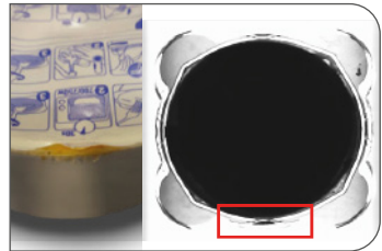
ACQUISITION EXAMPLE AND REAL DEFECTIVE PRODUCT
